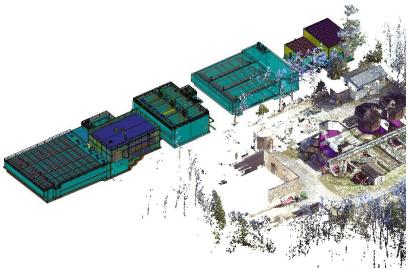
LIDAR or Point Cloud surveying produces a 3D point model. Through these points, the Plant 3D or Civil 3D designer can produce precise locations of existing piping and structures, creating a more accurate base than produced from record drawings, potentially saving on production time as well.
